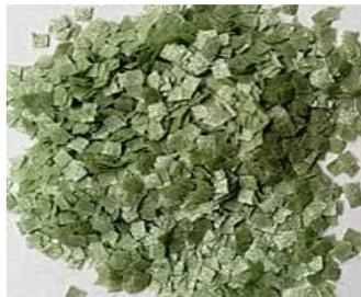
**ACTIFILMS™**AF is made up of Hydroxypropyl Methyl Cellulose which is a chemically modified cellulose polymer. HPMC is a water soluble synthetic polymer which was used as film former. It is a thin, flexible sheet of polymer in which an active ingredient has been incorporated. Actifilms rapidly disintegrate and also have greater stability and shelf life.
