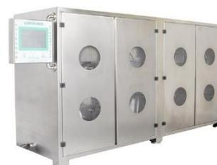
primary solution and further combining with secondary component to polymer solution. Secondary components such as active functional or decorative ingredients are finally deposited into the primary solution onto the casting surface for film formation using Umang Pharmatech's UCFC-600 (Solution tank ,Film Casting). The resulting solution is cast as a film and allowed to dry, which are then cut into pieces of the desired size and shape.
