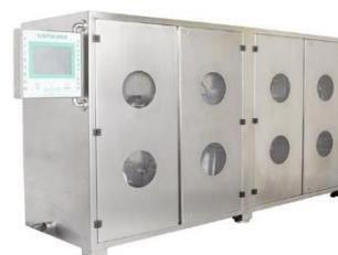
to polymer solution. Secondary components such as active functional or decorative ingredients are finally deposited into the primary solution onto the casting surface for film formation using Umang Pharmatech's UCFC-600 (Solution tank ,Film Casting). The resulting solution is cast as a film and allowed to dry, which are then cut into pieces of the desired size and shape.
